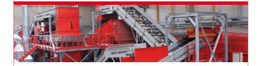
One of the typical sorting tasks which are built-in in our plant are sorting of polymers according to their type of material (PET, HDPE, PP, PS, mixed polymers, etc) and beverage cartons.
